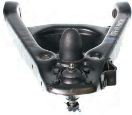
Lower Ball Joint install, facing down
