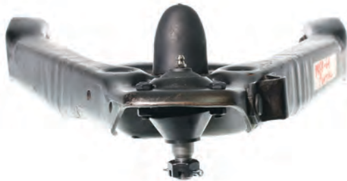
Lower Ball Joint installs from the bottom, facing down
